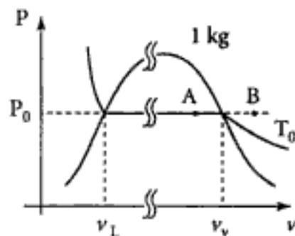
$$\text{Or } P_i = P_f = P_0 \quad \begin{cases} H_f = U_f + P_f V_f = U_f + P_0 V_f \\ H_i = U_i + P_i V_i = U_i + P_0 V_i \end{cases}$$
