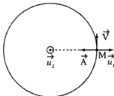
$$\text{Soit : } -m \frac{V_0^2}{a \sin \alpha_0} \vec{u}_r = -mg \vec{u}_z + R \vec{u}.$$
