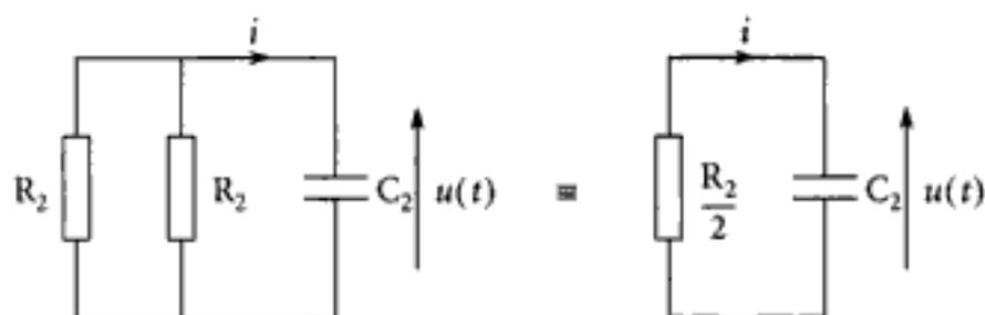
$$\text{Dès lors : } u = -\frac{R_2}{2}i \text{ et } i = C_2 \frac{du}{dt} \Rightarrow \frac{du}{dt} + \frac{2}{R_2 C_2} u = 0$$
