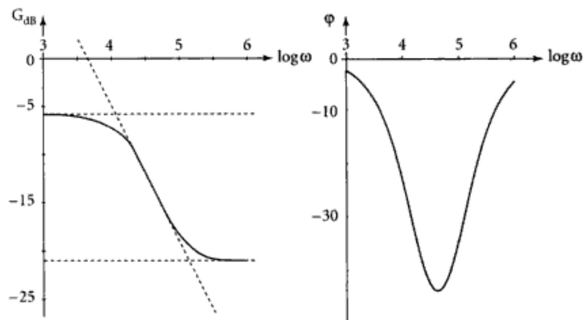
Ici,  $R_1 = 10 \text{ k}\Omega$ ;  $C_1 = 1 \text{ nF}$ ,  $C_2 = 10 \text{ nF}$  et on a pris:  $R_2 = R_1$ . On a alors  $\log \omega'_0 = 4,63$ .
