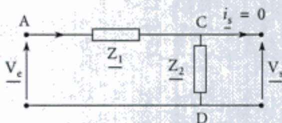
$$\text{Or } Y_2 = jC_2\omega \text{ et } Y_1 = \frac{1}{R_1} + jC_1\omega = \frac{1}{R_1}(1 + jR_1C_1\omega)$$
