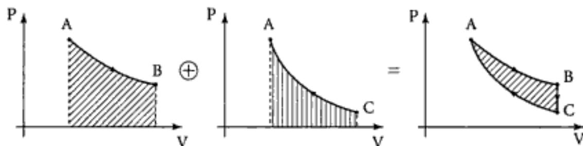
$$W(A \rightarrow B) = -\int_A^B P dV < 0 = W_1 \quad W(C \rightarrow A) = -\int_A^C P dV > 0 = W_2 \quad W_{\text{cycle}} = W_1 + W_2 < 0$$
