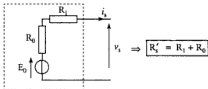
Mais  $R_0 = 50 \text{ }\Omega$  et  $R_1 = 10 \text{ k}\Omega$  soit  $R'_s = R_s = 10 \text{ k}\Omega$
