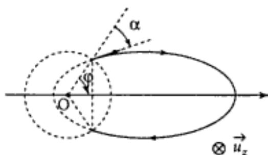
D'où  $\frac{p}{R} = 1 + e \cos(\pi - \varphi) \Rightarrow \cos \varphi = \frac{1 - \frac{p}{R}}{e} \quad (\theta = \pi - \varphi)$
