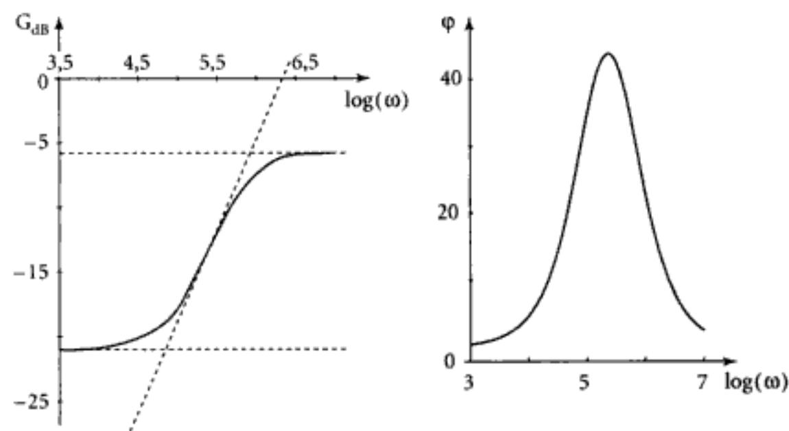
Ici,  $C_1 = C_2 = 1 \text{ nF}$ ;  $\frac{R_1}{R_2} = 10$  ( $R_1 = 10 \text{ k}\Omega$  et  $R_2 = 1 \text{ k}\Omega$ ) et  $\log \omega'_0 = 4,63$ .
