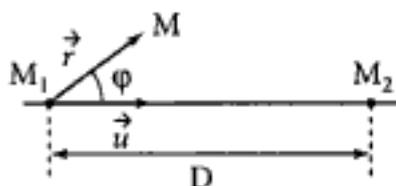
Soit encore :  $\delta\vec{G} = \frac{\mathcal{G}m_2}{D^2} \left\{ \frac{\left( \vec{u} - \frac{\vec{r}}{D} \right)}{\left\| \vec{u} - \frac{\vec{r}}{D} \right\|^3} - \vec{u} \right\}$  (1)
