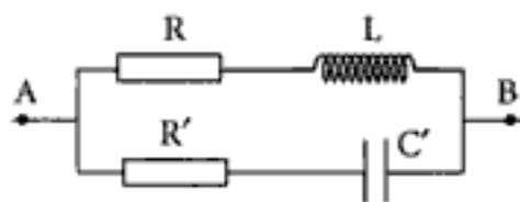
Or  $\underline{Y} = \underline{Y}_{RL} + \underline{Y}_{R'C'}$  (association en parallèle) et  $\underline{Y}_{RL} = \frac{1}{R + jL\omega} = \frac{1}{R \left(1 + j\frac{L\omega}{R}\right)}$ .
