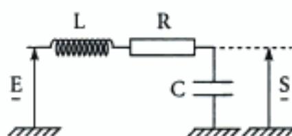
$$\bullet \omega \gg \omega_c \Rightarrow G_{dB} \sim -40 \log\left(\frac{\omega}{\omega_c}\right) = -40X \quad \text{avec} \quad X = \log\left(\frac{\omega}{\omega_c}\right)$$
